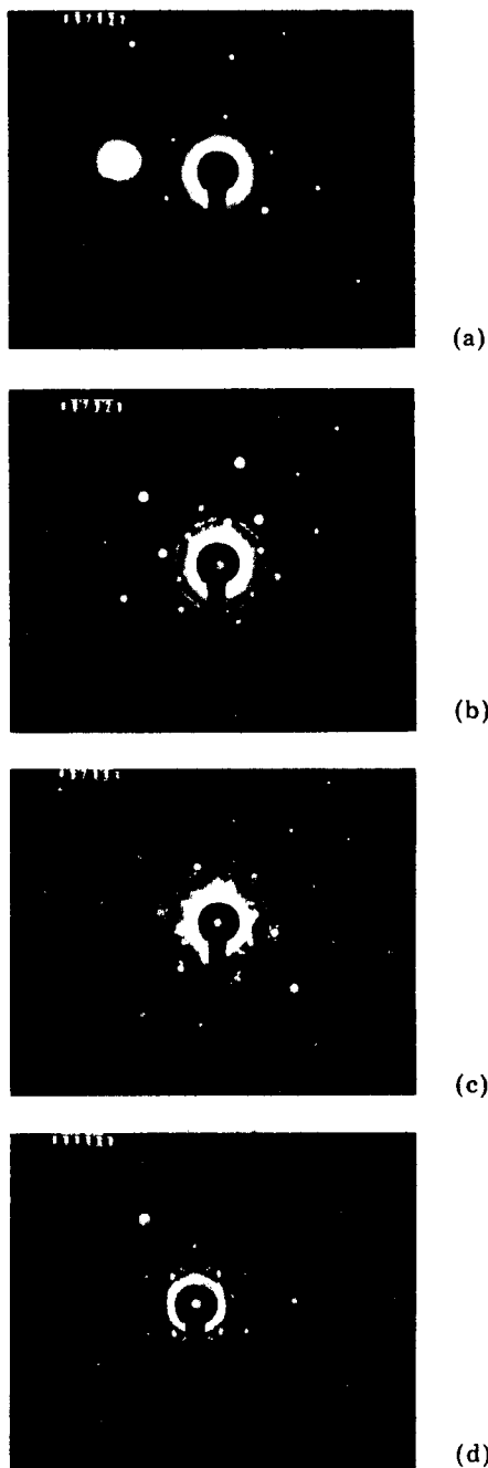
Fig. 8. Room temperature electron diffraction patterns for: (a) pristine graphite, (b) graphite- \text{Br}_2 , (c) graphite- \text{ICl} , (d) graphite- \text{IBr} .
